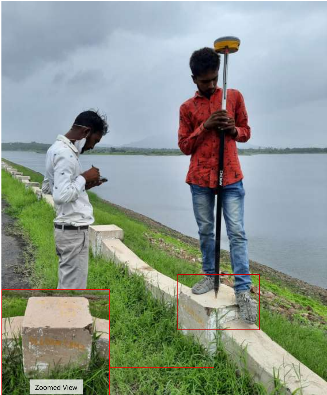
Figure 3.2: Temporary Benchmark (TBM2)
